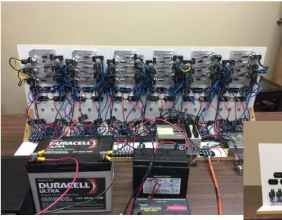
The test station as seen from the back which includes the bulbs and PLC and from the front with the relays and counters.
