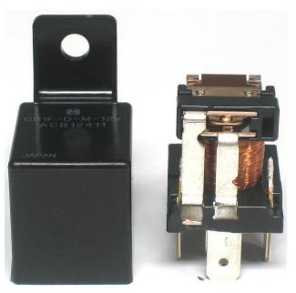
This next photo is of the Omron G8JN 40/30 automotive relay. The right hand view shows the two narrow beryllium copper springs that carry the entire power load. At least Omron put the relay contacts near the bottom of the relay. What is difficult to see is the narrow Strip of copper that goes from the normally open terminal up to the normally open contact. See the arrow.
