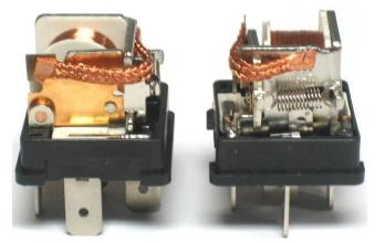
As a side note, the Aromat and Omron terminals are plated. But if you look closely, you can see copper on the edges of their terminals. They plate the material in the flat, then punch out and form the terminals. We plate our terminals after they are formed.
