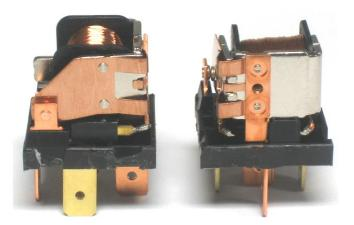
Finally here is our PC792A relay. Looks a little bit like the Tyco (Bosch) design, doesn't it? Below is the Tyco again for comparison. They only way to tell them apart, except for the resistor is that the Tyco terminals are unplated, while ours are nickel plated. We have sold over 4 million of these relays over the past few years and don't get any back.
